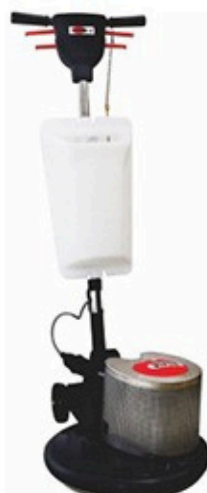
AN 17SC 石材处理机 AN 17SC Stone processor 电压/Voltage (V): 220~240 功率/Power (W): 1500 电线长度/Cord length (m): 15 转速/Speed (rev/min): 160 底盘直径/Chassis Diameter (cm): 43 规格/Size (cm): 62x47x132 重量/Weight (kg): 70
