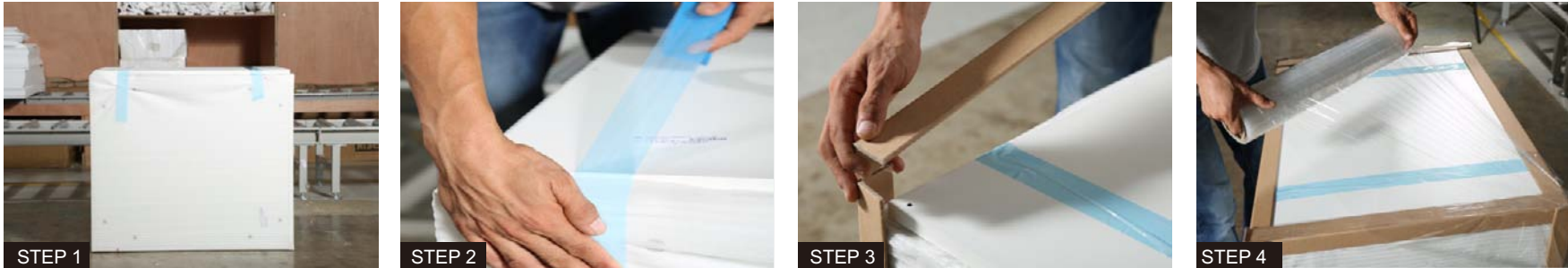
STEP 1 Wrap each cabinet completely with EPE film, no exposures. STEP 2 Fix EPE film with blue tapes. STEP 3 Protect edges with cardboard edge protectors STEP 4 Tightly wrap the cabinet with stretch film.
