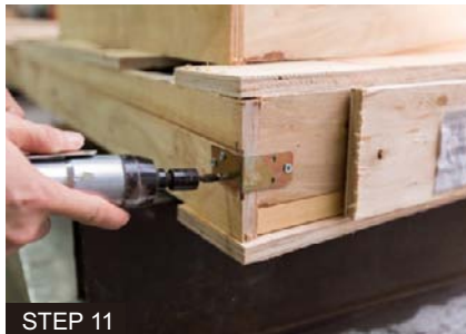
STEP 11 Nail the metal corners onto side slats
