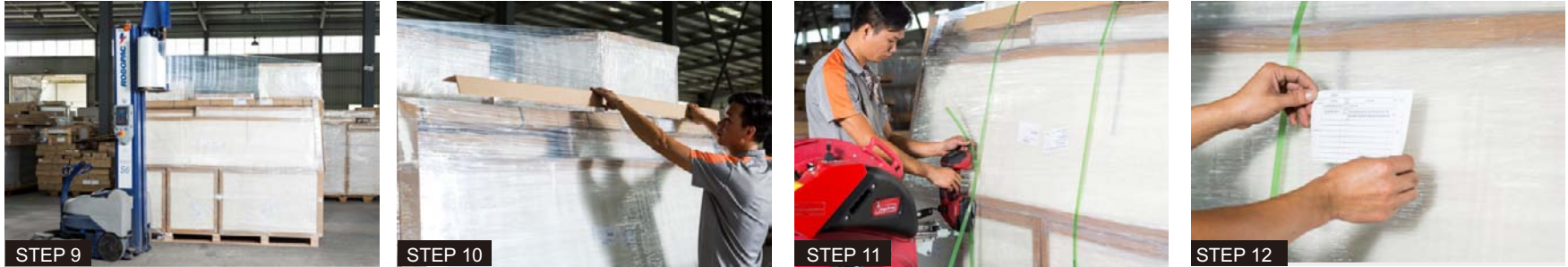
STEP 9 Tightly wrap all units with stretch film. STEP 10 Cover the top edges with cardboard edge strips, then fix them with tape. STEP 11 Tighten the palletized units with plastic belts. 4 belts in horizontal direction and 2 belts in vertical direction. STEP 12 Label the pallet with shipping mark. The shipping mark can be specified.
