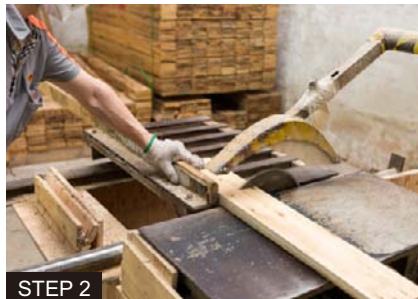
STEP 2 Cut slats to size according to the countertop size. The longer pieces will be the sides of your crate and the shorter boards will be the ends.
