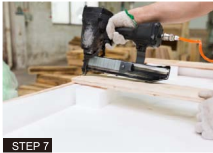
STEP 7 Attach front rails to side slats with the nail gun.
