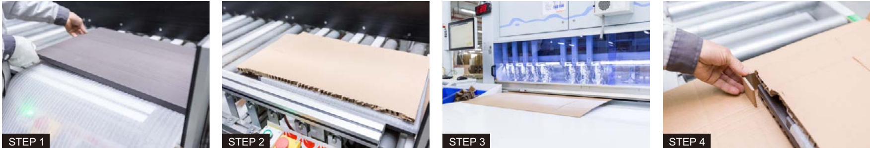
STEP 1 Wrap each panel with EPE foam, no exposures STEP 2 Cover each panel with honeycomb paper STEP 3 Cut carton based on panel dimensions STEP 4 Protect each panel with edge protectors.
