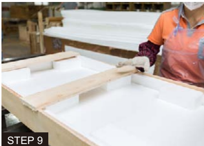
STEP 9 Attach back rails to side slats with the nail gun.
