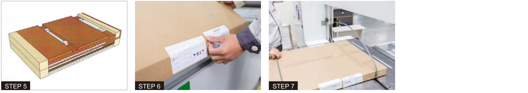
STEP 5 Stack packed panels into eight layers; and place the slide box at the left side and hardware box at the right side. STEP 6 Cover the stack with carton and label it. STEP 7 Tighten the carton with belts
