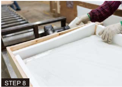
STEP 8 Turn the countertop and box over, then fill the back voids with foam boards.
